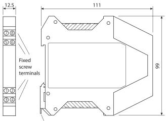
Metal interlock to attach to mounting rail
